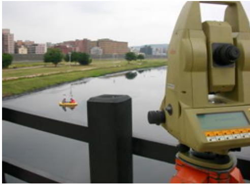
Fig. 2 Channel survey work on No Name Creek
